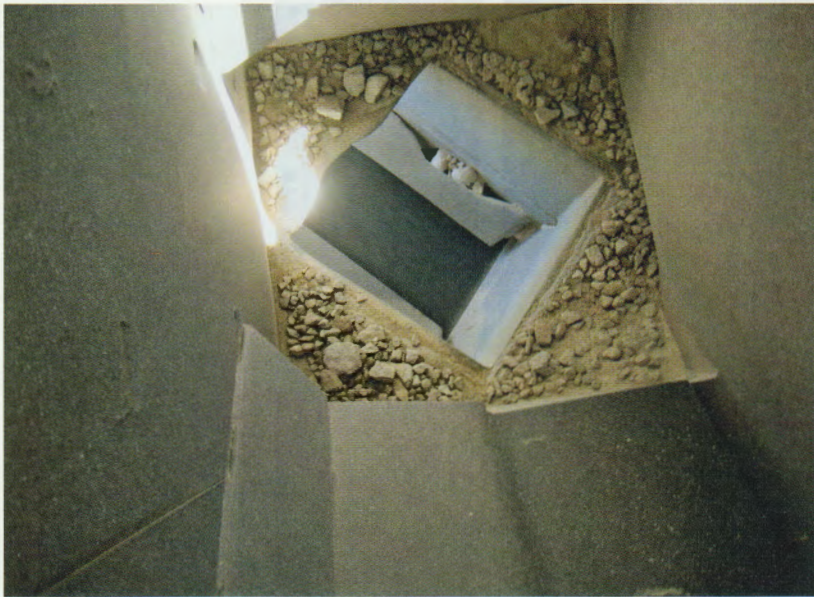
A rock box acts like a shelf, catching and distributing falling material onto the impact cradle
